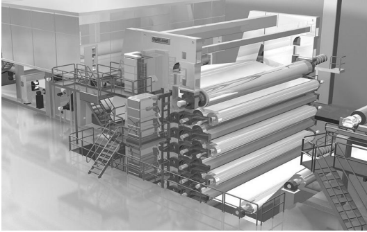
Fig. 15. An OptiLoad multinip calender can be added to an existing paper machine online or offline.
