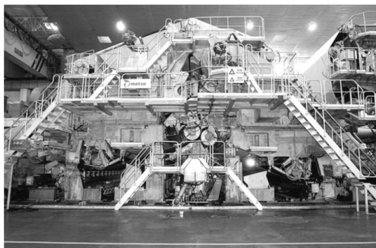
Fig. 18. The original BelBaie III former was upgraded to a BelBaie V, which extends the former's life to match the latest modern machines.
