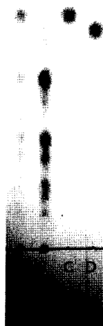
Fig. 6. Thin layer chromatography of the reaction product hydrolyzed by the amylolytic enzyme of S. cerevisiae HA 27 in soluble starch. The product of hydrolysis by the amylolytic enzyme of S. cerevisiae HA 27 (A), maltooligosaccharide (B), glucose (C), maltose (D).
