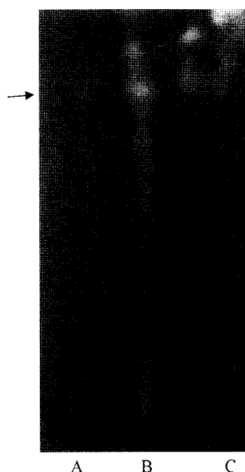
Fig. 2. TLC analysis of standard taxol (A) and fungal taxol from M1D (B), and PDB (C) in silica gel pre-coated aluminium sheet. Arrow mark indicates the presence of taxol spot in all the 3 samples illuminated with UV at 254 nm.
