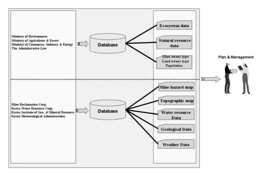
Fig. 2. GIS Concept Diagram for Planning and Management.
