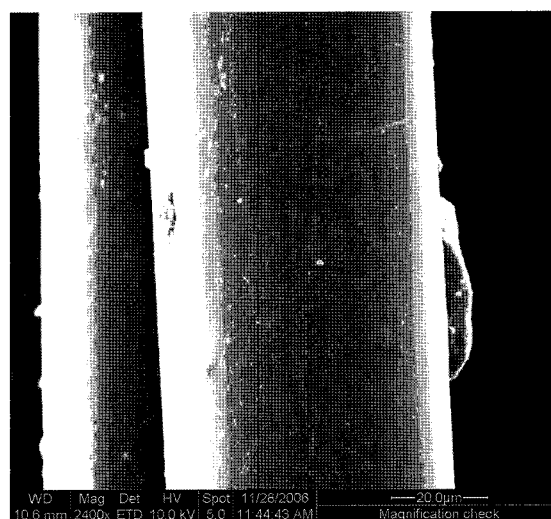
Figure 19. SEM image of the sheath-core bicomponent composite fiber.
