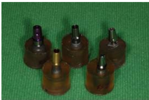
Fig. 1. Samples which were mounted in liquid unsaturated polyester.
