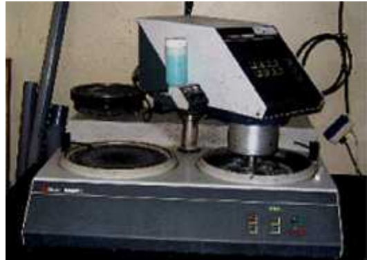
Fig. 3. Automatic specimen polisher (Rotopol 2, Struers, Denmark).
