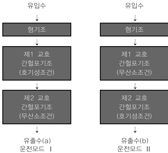
Fig. 3. Operation condition of 2 stage IA process.
