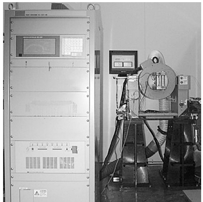
Fig. 2 System for evaluating anti-vibration gloves' performance
