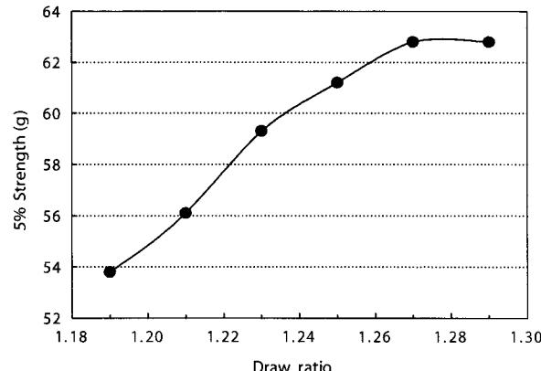
Fig. 11. 5% Strength of textured yarn as a function of draw ratio.
