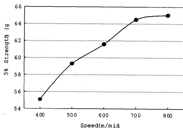
Fig. 4. 5% strength of textured yarn a function of speed.
