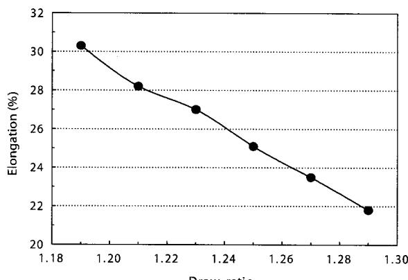
Fig. 13. Elongation of textured yarn as a function of draw ratio.
