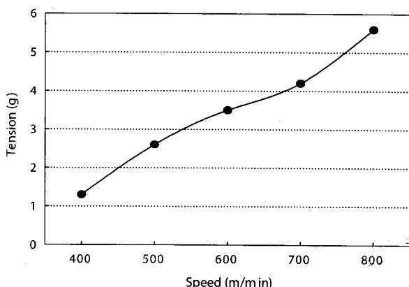
Fig. 2. Unwinding tension as a function of speed.
