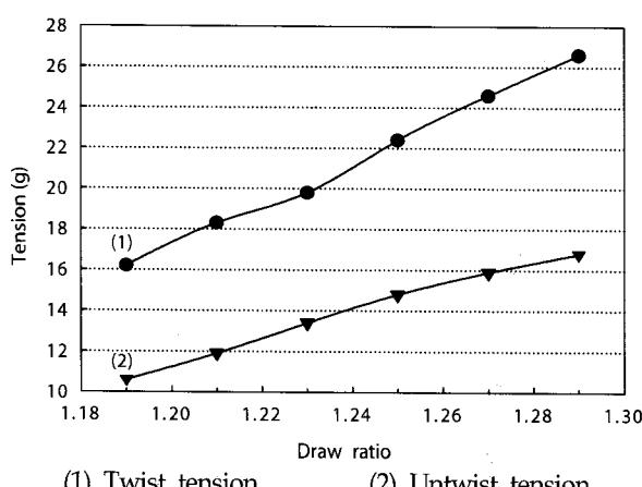
Fig. 9. Twist and untwist tensions as a function of draw ratio.
