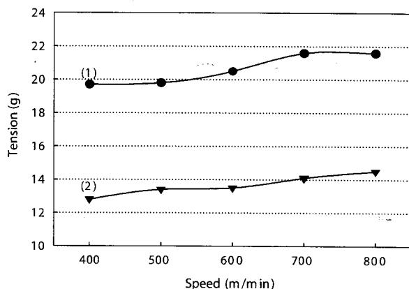
Fig. 1. Twist and untwist tensions as a function of speed.
