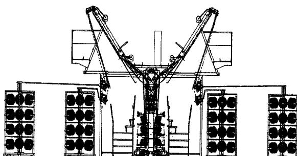
Scheme 2. Schematic false twist machine of Barmag FK-6.
