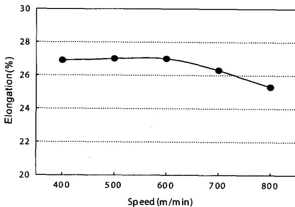
Fig. 5. Elongation of textured yarn as a function of speed.
