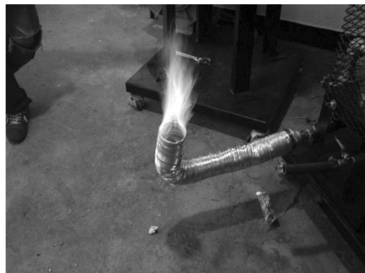
Fig. 3 Flame of producer gas from charcoal gasification
