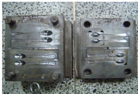
Fig. 5 Experimental mold
