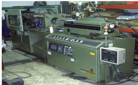
Fig. 4 Injection molding machine used for experiment
