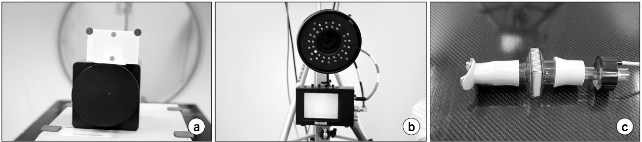
Fig. 1. Equipment of respiratory signal : Varian RPM system :(a) Moving phantom and reflective marker, (b) Components of RPM respiratory gating system, (c) Turbine type spirometer.
