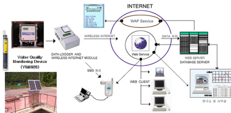
Fig. 2. Configurations of Real Time Data Acquisition and Wireless Communication System of RTMMS
