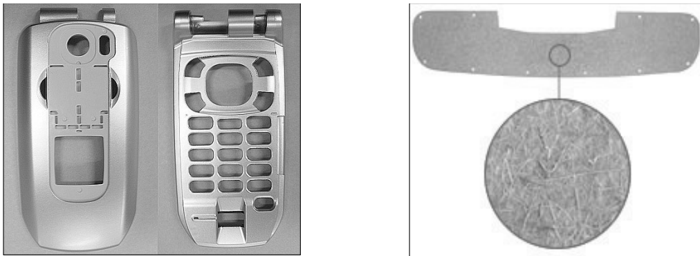
Fig. 1. Practical using of bio-composite reinforced with natural fibers.(Housing of mobile phone and interior materials of automobiles.)
