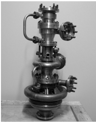
Fig. 2 10-ton class LOX-LCH4 turbopump
