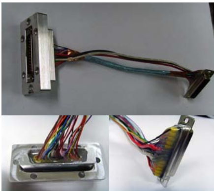
Fig. 5 Complete Unit of Vacuum Connector
