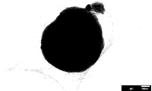
Fig. 4 TEM micrograph of a Fe-coated particle.
