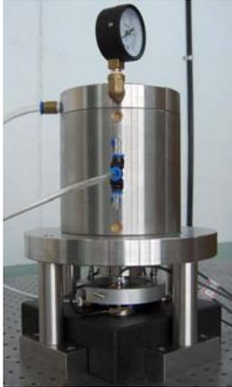
Fig. 3 Entire experimental setup for measuring load and gap.
