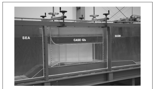
Fig. 3 A model of sluice caisson and mound installed in the open channel flume.
