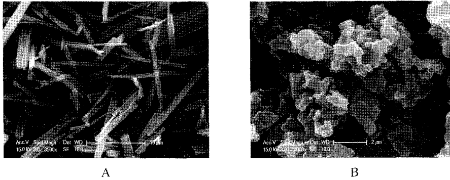
Figure 2—SEM micrographs of paclitaxel raw material, 3500× (A) and paclitaxel solid dispersion, 10000× (B).
