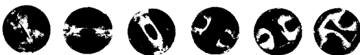
Fig. 6 Experimental smoked-foil records for two-cell detonation mode in a round tube' wall and front-end, by Penyazkove and Sevrouk 2 .
