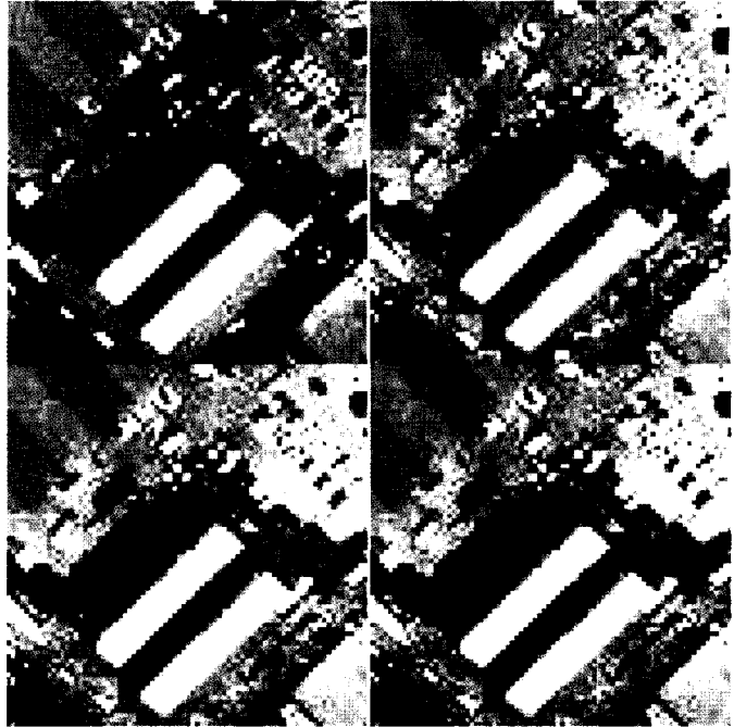
Fig. 3. Results of sharpening process to remove block distortion(original panchromatic image and FitPAN-fused image before sharpening process in the top line, FitPAN-fused images after sharpening process of 7 \times 7 window with r = 0.5 and 2.0 respectively from left in the bottom line).
