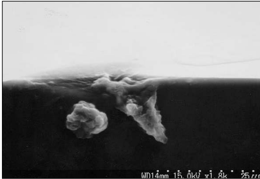
[그림 8] A cross section to cut a hole by corona discharge treatment. Magnified X1,800
