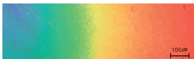
Figure 2. Photomicrograph the CLC film with the induced pitch gradient covering from blue to red pitches at RT.
