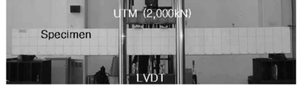
Fig. 2 Setup of loading (mm)
