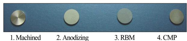
**Fig. 1.** Surface treated disc.
