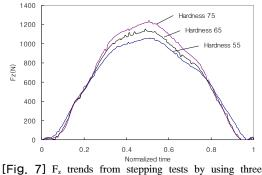
[FIG. 7] F<sub>z</sub> trends from stepping tests by using three different hardness specimen shoes.
