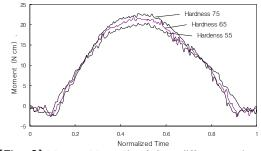
[Fig. 9] Moment M<sub>x</sub> trends of three different specimen shoes
