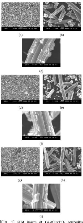
[Fig. 1] SEM images of Co-ACFs/TiO<sub>2</sub> composites prepared with TNB and cobalt chloride modified ACFs;
