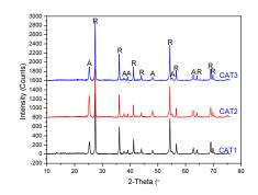
[Fig. 2] XRD patterns of Co-ACFs/TiO<sub>2</sub> composites prepared with TNB and cobalt chloride modified ACFs with heat treatment at 973 K for 1 h.
