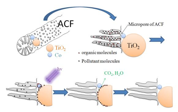
[Fig. 5] Schematic illustration of adsorption, photocatalysis and regeneration of Co-ACFs/TiO<sub>2</sub> catalyst.
