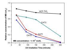
[Fig. 4] Dependence of relative concentration of MB in the aqueous solution c/c0 on time of UV irradiation for the Co-ACFs/TiO<sub>2</sub> composites prepared with TNB and cobalt chloride modified ACFs.
