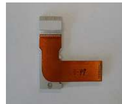
Fig. 6 16 Channel Si photodiode coupled to CdWO 4 crystal
