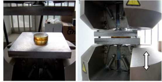
Fig. 5 Uniaxial compression test of urethane using material test machine
