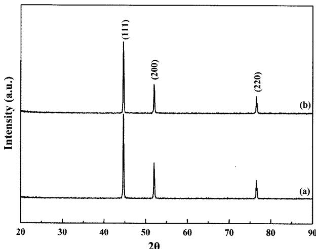
Fig. 9. The XRD pattern of Ni phase formed by reduction of NiO nano crystals 5%H<sub>2</sub>/N<sub>2</sub> atmosphere. (a) at 600°C for 15 minutes and (b) at 600°C for 60 minutes.
