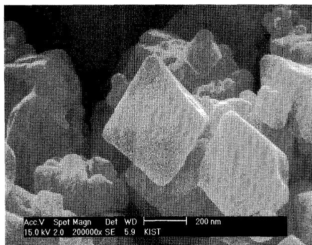
Fig. 2. SEM micrograph of  $\text{NiO}$  nano crystals synthesized by heat treatment at  $500^\circ\text{C}$  for 5 hours.
