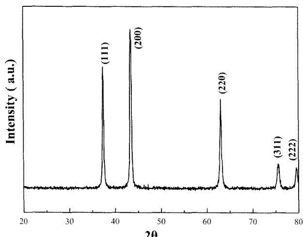
Fig. 1. The XRD pattern of the  $\text{NiO}$  nano crystals obtained by heat treatment of  $\text{Ni}(\text{NO}_3)_2 \cdot 6\text{H}_2\text{O}$  at  $500^\circ\text{C}$ .
