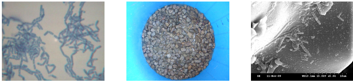
Fig. 2. Bacillus subtilis (×1,000)(L), Seeding pumice stone and recycled aggregate(C) and SEM(×5k)
