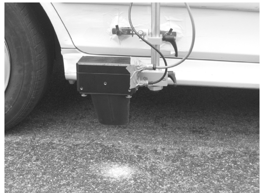
Fig. 2 Non-contact optical sensor(speedometer)
