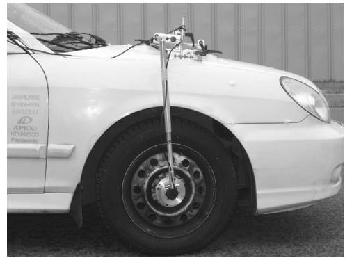
Fig. 3 Attachment of wheel rotation speed sensor
