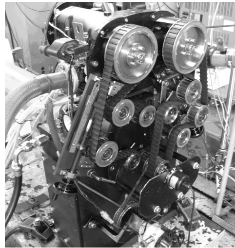
Fig. 1 MCVVT system for the hydrogen-fueled engine.
