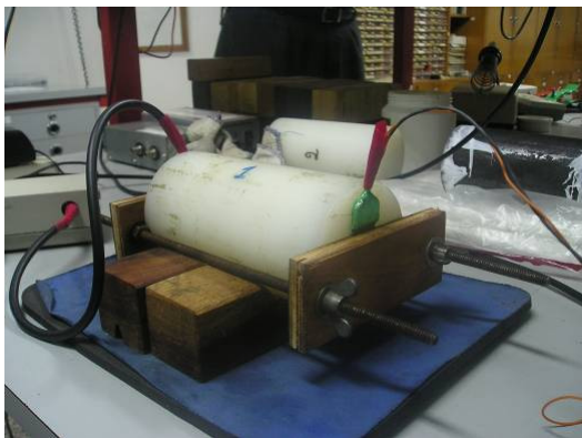
Fig. 5 Nylon test cylinder with the emitter and receiver PVDF transducers in both sides of the cylinder
