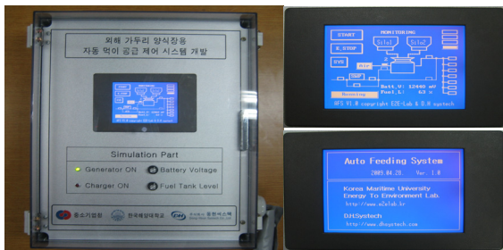
Fig. 7 Photograph of Auto feed control system.
