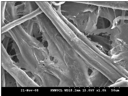
Photo 3. SEM of bamboo BKP sheet.
