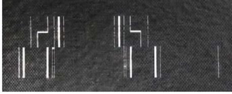
Fig. 11 The prepreg with slots after laser cutting.
