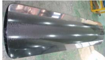
Fig. 13 Completed Composite Cradle.
