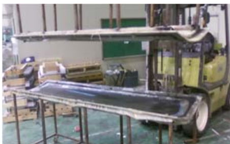
Fig. 11 Assembly of Upper mold and Lower mold.
