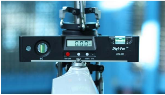
Fig. 10. Correction of Collective Pitch Angle
