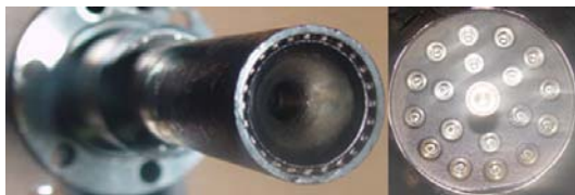
Fig. 7. Baffle injector installed at the center of subscale combustor head
