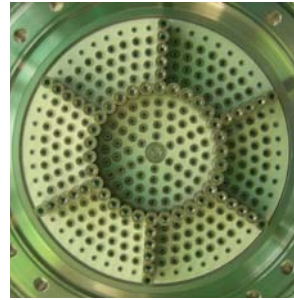
Fig. 12. Arrangement of injectors in full-scale combustor mixing head
