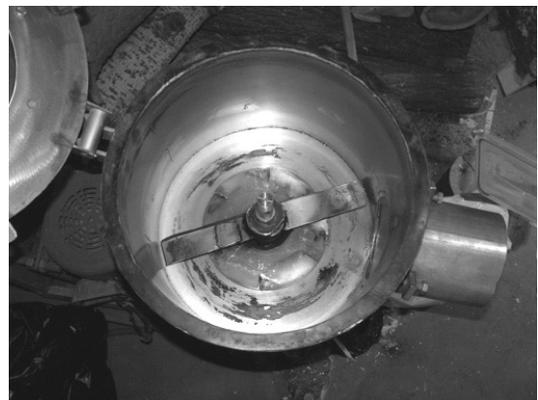
Fig. 1. Dry disintegrator with two rotors.
