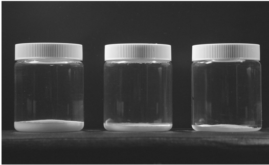
Fig. 7. Images of T-FWA at concentrations of 0.05(left), 0.03(middle), 0.01 (right) % controlled to pH 4.7 with alum.
