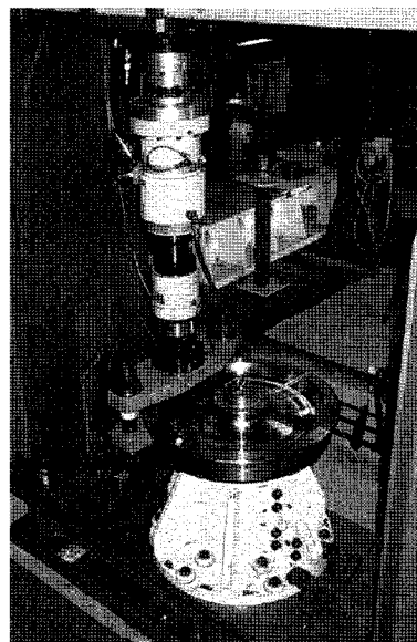
Photo 4 Wheel fatigue test
