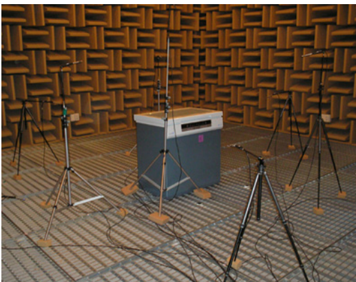
Fig. 1 Measurement of the sound power level in the semi-anechoic room
