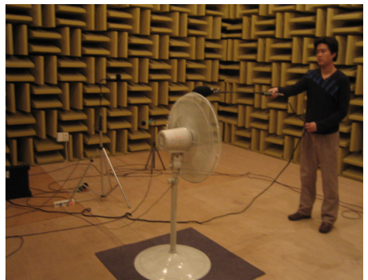
Fig. 3 Measurement of the sound power level by intensity method
