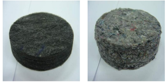
Fig. 2 Examples of layered structure of specimen(left picture : PET, right picture : Resin Felt)
