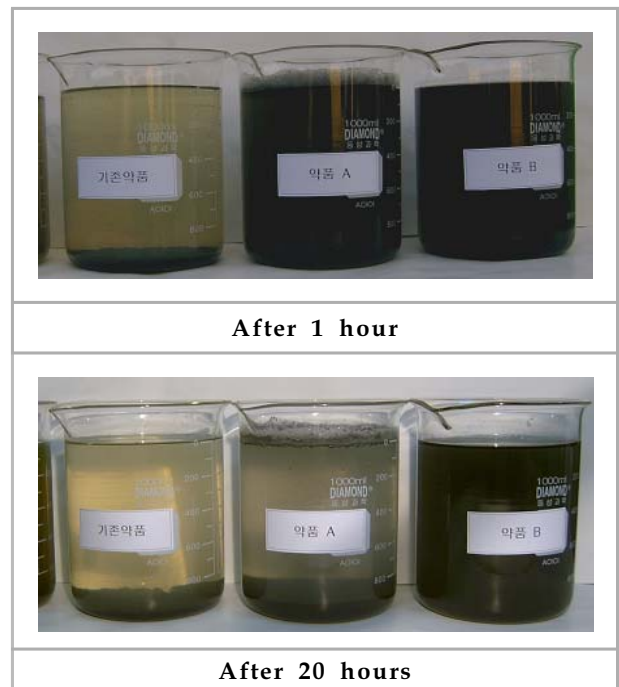
Fig. 10. Comparison of turbidity between samples treated by 3 kinds of coagulants with the lapse of time (1 hour and 20 hours) after agitation and settlement.
