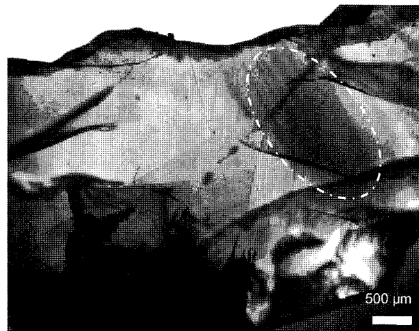
Fig. 2. The presence of the dense cloudy brownish tiny particles near the former dark blue core region.
