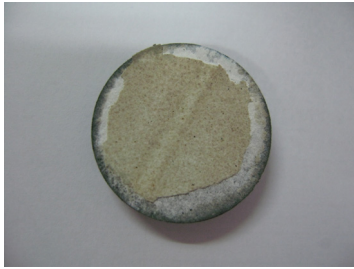
Fig. 9 Partial separation of coating layer from substrate (80 cycles)
