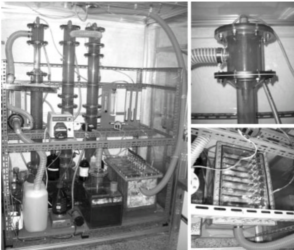
Fig. 5. Hybrid VOCs treatment system.
